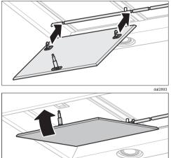
Hook the panels onto the support ledge, lift up the front and push them into the lock until they engage.
